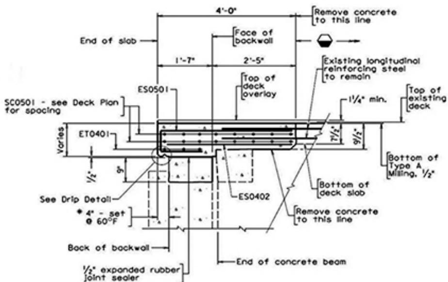
Fig. 5. Detail for "Deck Extension" Eliminating Joint at Abutment
