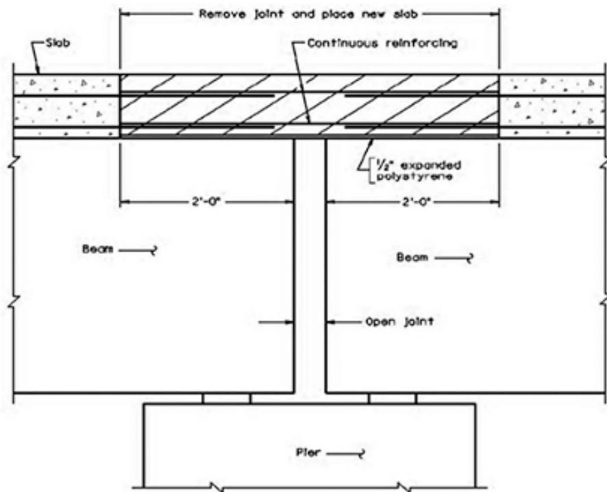
Fig. 4. Detail for "Link Slab" Eliminating Joint over Pier
