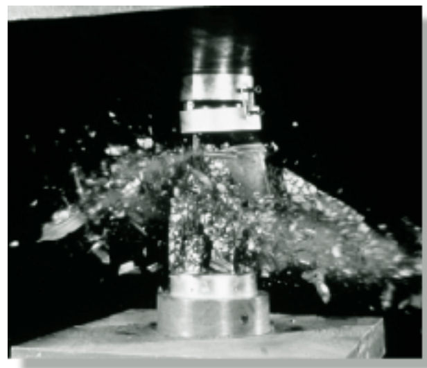
Compression testing of high strength concrete requires special care.
