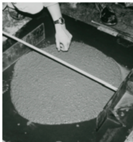
Fig. 2 Measuring slump flow consistency
