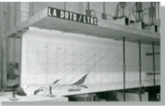
Shear test of 72-in. (1.83-m) deep bulb-tee girder.
