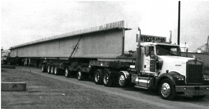
High strength concrete was used in the largest girders shipped in Washington State.
