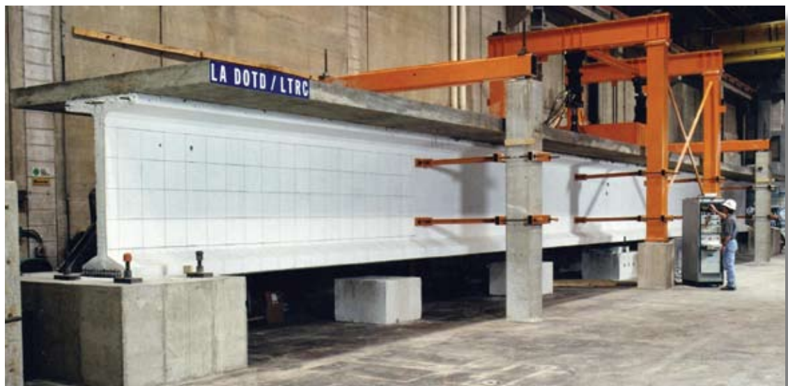
Fatigue testing of full-size HPC girder.
