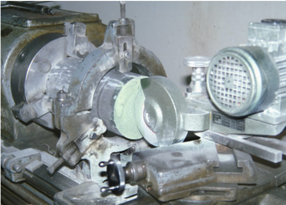
Grinding a high strength concrete cylinder.
