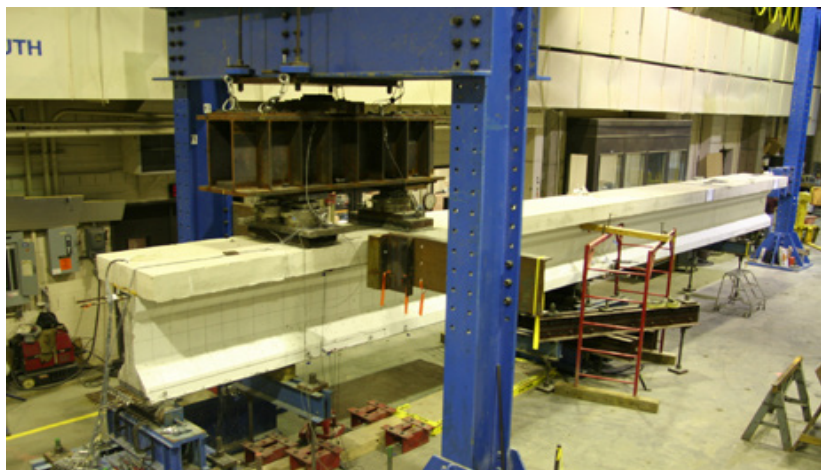
Strand development length test of LWHPC
