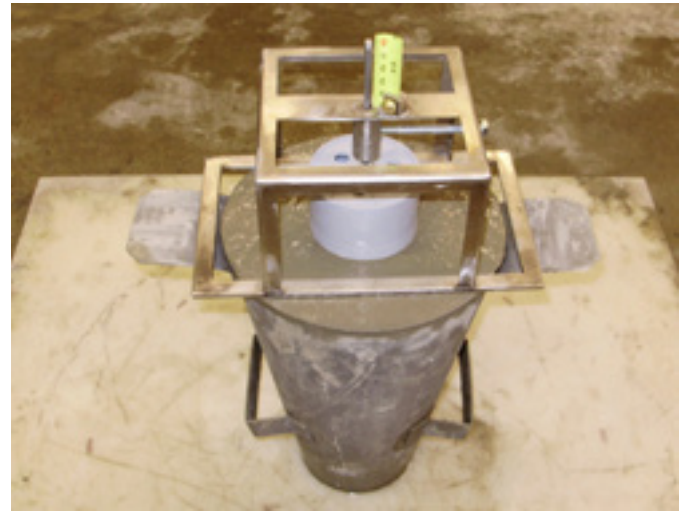
Apparatus used in ASTM C1712. Photos: BASF
