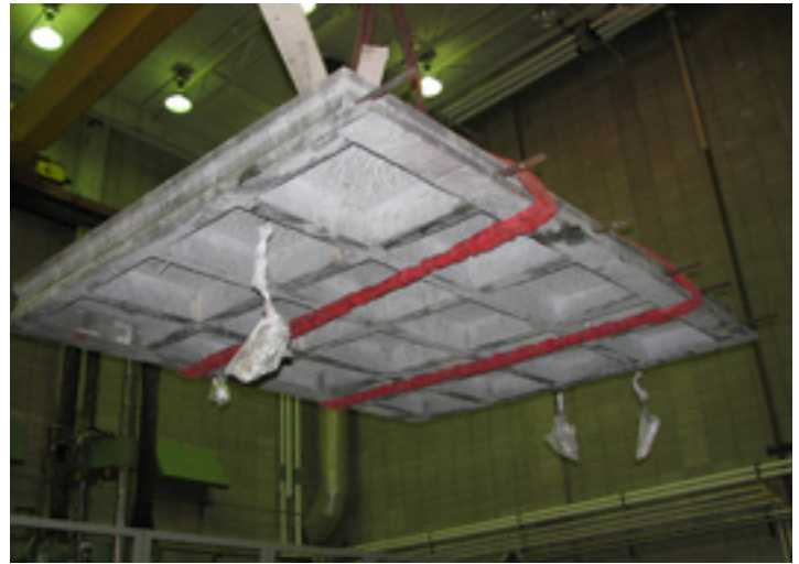
Full scale laboratory tests of the waffle slab system were performed.
