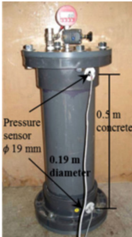
Pressure device to simulate SCC formwork pressure.
