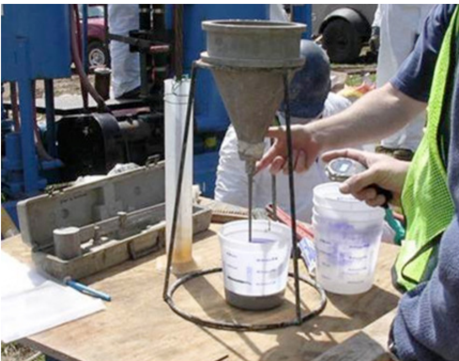
Fig. 2. The wet density and flowability are tested at mixer as well as at the the outlet
