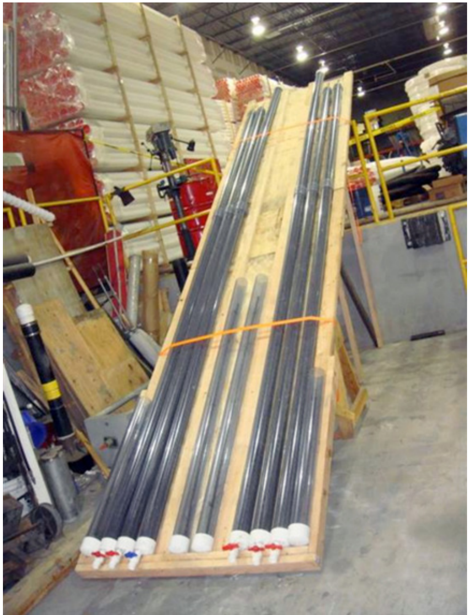
Fig. 1. The inclined tube test is a large scale bleed test. Photo: Structural/VSL
